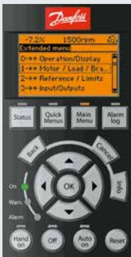
VLT® and VACON® drives feature a user-friendly, hot pluggable local control panel (LCP) for easy setup and parameter configuration.
